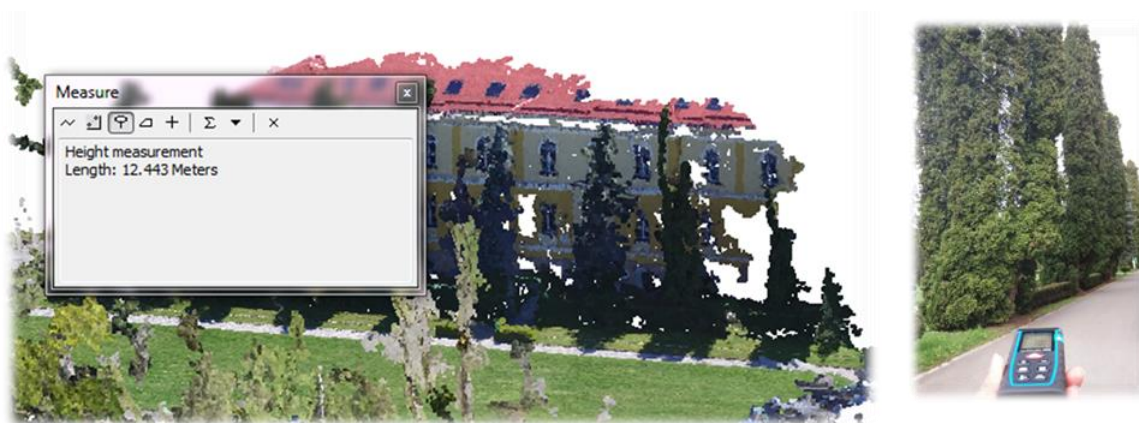
Fig. 9 The estimation of tree height using the point cloud and validation with telemeter and forestry caliper
